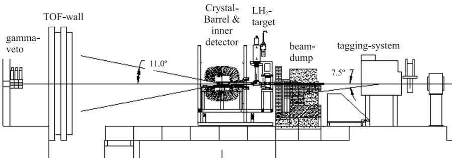
Fig. 1. Setup of the CB-ELSA detector during the first data taking period.
