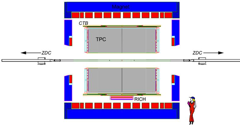
Fig. 1. Cross-sectional view of the STAR detector.
