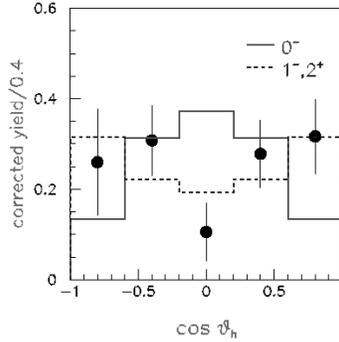
Fig. 10. The efficiency-corrected  $D_{sJ}(2458)^+$  yield as a function of  $\cos \theta_h$ . The solid [dashed] histogram corresponds to a  $\sin^2 \theta_h$  [ $(1 + \cos^2 \theta_h)$ ] distribution.
