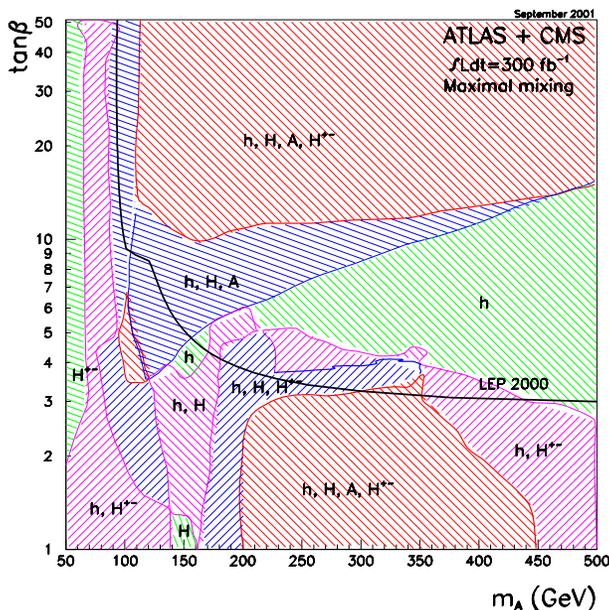
Fig. 6. The combined sensitivity of the ATLAS and CMS experiments for the discovery of MSSM Higgs bosons (in the case of maximal mixing). The excluded regions with a significance of  $5\sigma$  in the  $(m_A, \tan\beta)$  plane are shown. In the different regions the number of supersymmetric Higgs bosons that can be detected is indicated. Also included are the limits obtained from the LEP2 data.
