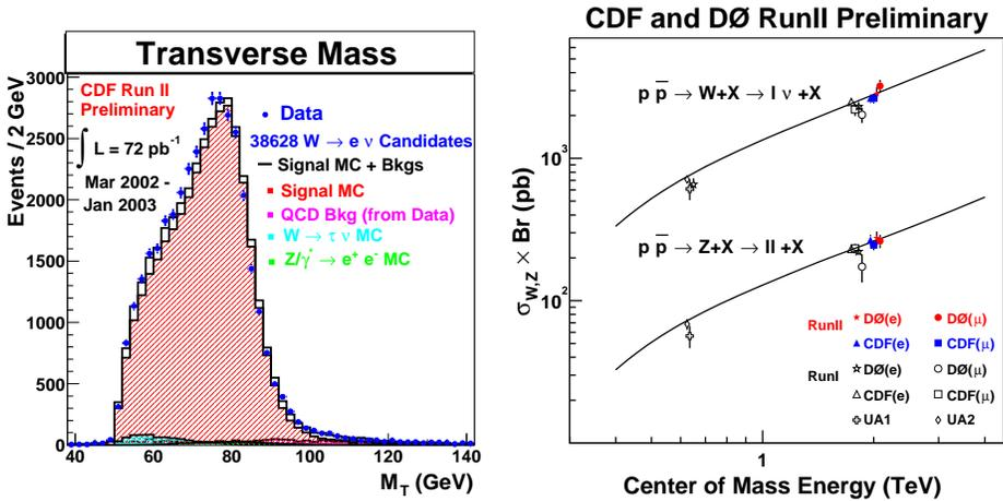
Fig. 2. (left): The transverse mass distribution of the  $W \rightarrow e\nu$  candidates selected in the CDF Run II data based on an integrated luminosity of  $72 \text{ pb}^{-1}$ . (right): The  $W$  and  $Z$  boson production cross section as measured in the CDF and DØ in Run I and from first data collected in Run II. The NNLO QCD predictions are superimposed.
