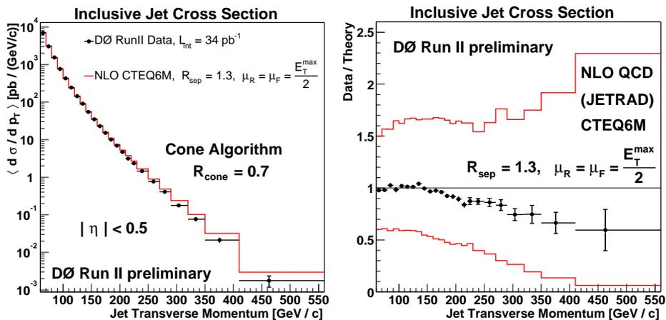
Fig. 1. (left): The inclusive jet production cross section as a function of  $P_T$  from data collected in the D0 experiment in Run II. The QCD prediction is superimposed. (right): Ratio between the experimental data and the theoretical predictions. The band indicates the systematic uncertainties in the data resulting from the uncertainties on the absolute jet energy scale.
