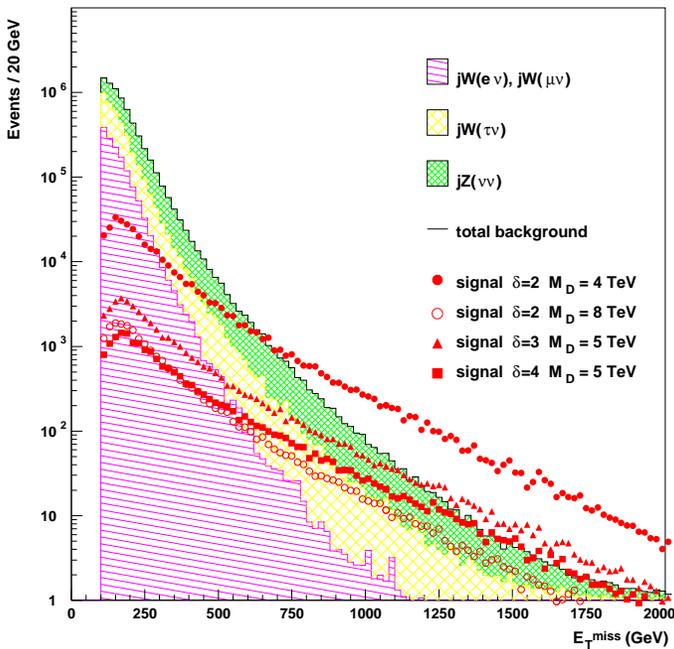
Fig. 12. Distribution of the missing transverse energy in background events and in signal events after the selection and for  $100 \text{ fb}^{-1}$ . The contribution of the three main kinds of backgrounds are shown as well as the distribution of the signal for several values of  $(\delta, M_D)$ .
