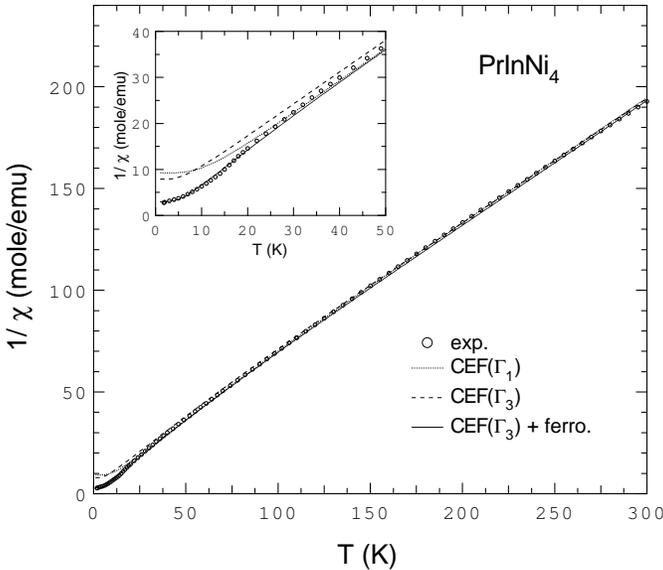
Fig. 1. The temperature dependence of  $1/\chi$ . The dots, dashed and solid lines represent the calculated results obtained by considering CEF with  $\Gamma_1$  ground state ( $\Gamma_1$ ), CEF ( $\Gamma_3$ ) and CEF ( $\Gamma_3$ ) + ferromagnetic interaction, respectively. For the CEF level schemes used in the calculation, see the text.
