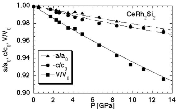
Fig. 1. Pressure dependence of  $a/a_0$ ,  $c/c_0$ , and  $V/V_0$  of  $\text{CeRh}_2\text{Si}_2$ . The solid line for the pressure dependence of  $V/V_0$  shows the result of Murnaghan's fitting. The dashed lines for  $a/a_0$  and  $c/c_0$  are guides to eye.
