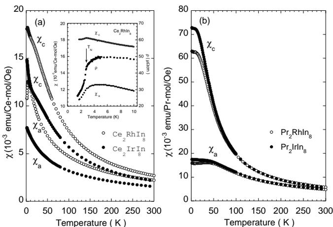
Fig. 1. Magnetic susceptibility for  $Ce_2MIn_8$  (a) and  $Pr_2MIn_8$  (b), where  $M=Rh$  and  $Ir$ . The inset in (a) presents temperature dependence of susceptibility and electrical resistivity at low temperatures.
