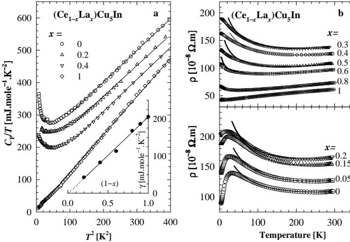
Fig. 1. (a) Specific heat of  $\text{Ce}_{1-x}\text{La}_x\text{Cu}_5\text{In}$ , and concentration dependence of the  $\gamma$ -coefficient (inset). (b) Electrical resistivity of  $\text{Ce}_{1-x}\text{La}_x\text{Cu}_5\text{In}$ . Solid lines indicate fits as described in the text.
