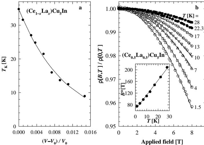
Fig. 2. (a) Volume dependence of the Kondo temperature  $T_K$  for  $\text{Ce}_{1-x}\text{La}_x\text{Cu}_5\text{In}$  observed experimentally (points) and fitted to the compressible Kondo model (line). (b) Magnetoresistivity of  $\text{Ce}_{0.5}\text{La}_{0.5}\text{Cu}_5\text{In}$ . The experimental data are fitted to the single-ion spin-1/2 Bethe ansatz description (see text).
