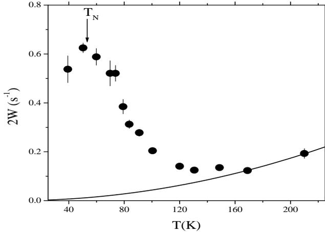
Fig. 2. Temperature dependence of  $^{139}\text{La}$  NQR spin-lattice relaxation rate in  $\text{La}_2\text{Cu}_{0.7}\text{Mg}_{0.3}\text{O}_4$ . The solid line shows the phonon contribution to the relaxation.
