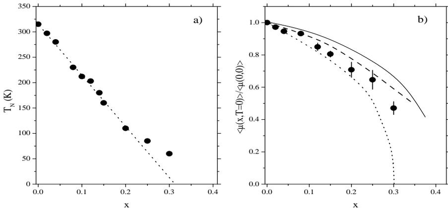
Fig. 1. (a) Néel temperature in  $\text{La}_2\text{Cu}_{1-x}(\text{Mg,Zn})_x\text{O}_4$ . The dotted line is the behavior expected within the dilution model. (b) Sublattice magnetization as a function of spin dilution. The solid line was derived from quantum Monte Carlo simulations [6], the dashed line from spin-wave theory [7], the dotted line in the framework of an effective quantum non-linear  $\sigma$  model [8].
