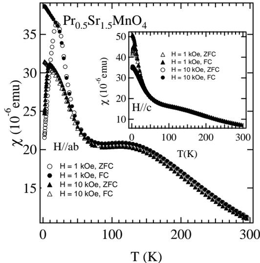
Fig. 1. ZFC and FC magnetic susceptibility as a function of temperature for  $\text{Pr}_{0.5}\text{Sr}_{1.5}\text{MnO}_4$  ( $x = 0.5$ ) compound for  $H||ab$  and  $H||c$  (inset) at two different applied fields,  $H = 1$  kOe and 10 kOe.
