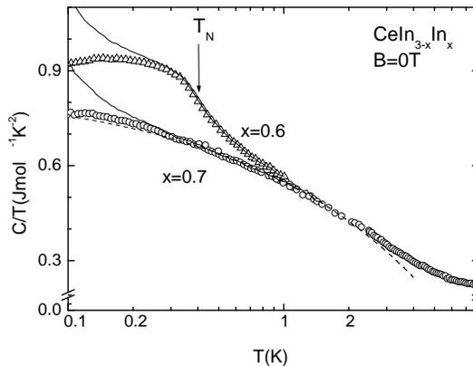
Fig. 2. Electronic specific heat of  $CeIn_{2.4}Sn_{0.6}$  ( $\Delta$ ) and  $CeIn_{2.3}Sn_{0.7}$  (O) plotted as  $C/T$  versus  $\log T$ . The solid lines show the experimental data. Symbols present the data after subtraction of a nuclear contribution which has been estimated from the data below 0.1 K (see text). The dashed line is a  $C(T)/T \propto \gamma_0 - b\sqrt{T}$ -fit through the data.
