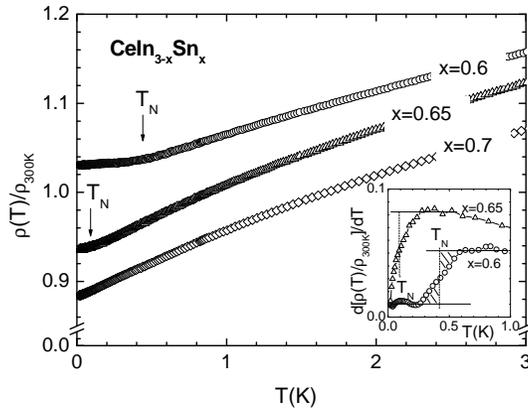
Fig. 1. Low-temperature zero field resistivity  $\rho(T)$  versus temperature of  $\text{CeIn}_{3-x}\text{Sn}_x$  with  $x = 0.6, 0.65$  and  $0.7$ . The arrow marks the Néel temperature estimated from an equal areas construction as shown in the inset.
