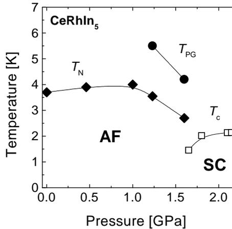
Fig. 2.  $P$ - $T$  phase diagram for CeRhIn<sub>5</sub>. The open marks are determined from ac-susceptibility measurement [10].
