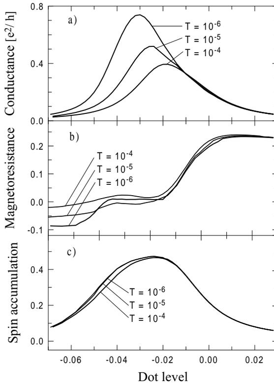
Fig. 1. The conductance (a), the magnetoresistance (b) and the spin accumulation (c) as a function of the position of the dot level for different temperatures  $T = 1 \times 10^{-6}$ ,  $1 \times 10^{-5}$  and  $1 \times 10^{-4}$ . The conductance and the spin accumulation are determined for the parallel configuration of magnetization.
