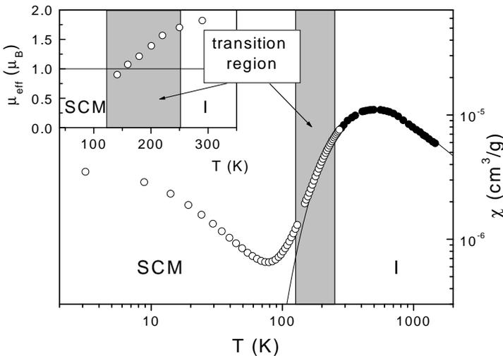
Fig. 1. Magnetic susceptibility of FeSi in a wide temperature range. Inset shows the temperature dependence of the effective magnetic moment  $\mu_{\text{eff}}$  of charge carriers. The Mott–Hubbard type MIT range is also shown (I — insulator, SCM — strongly correlated metal).
