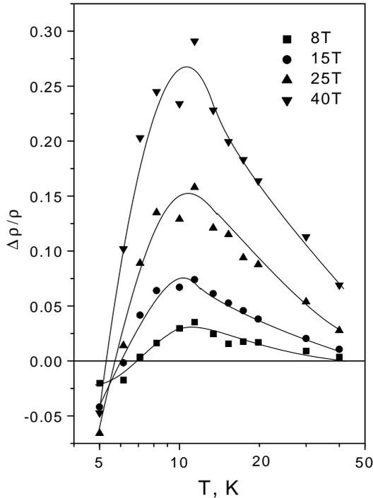
Fig. 2. Magnetoresistance of FeSi in steady (8T) and pulsed magnetic fields.
