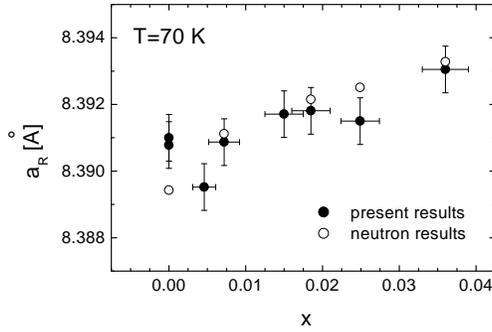
Fig. 2. Compositional dependence of rhombohedral lattice parameter  $a_R$  at  $T = 70$  K.
