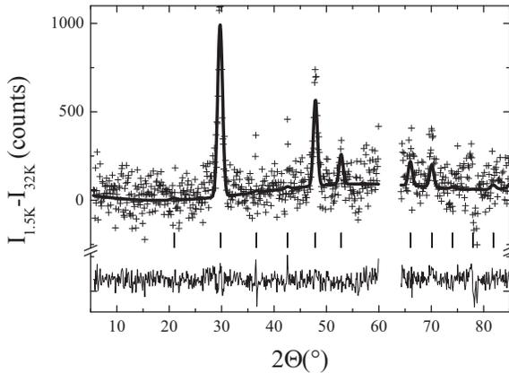
Fig. 2. The magnetic Bragg intensity  $I_{1.5 \text{ K}} - I_{32 \text{ K}}$  of  $UPd_{1.85}Sn$ . The data (+) is refined (solid line) assuming the structure from Fig. 3. Bragg peak positions are indicated by ticks, the solid line in the lower panel represents the difference between fit and data. The area of the main structural Bragg peak at  $62^\circ$  is omitted.
