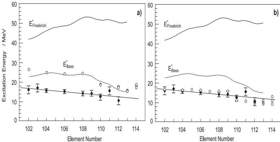
Fig. 17. The minimal excitation energy of the compound nuclei of 102–114 elements in cold fusion reactions ( $HI,1n$ ); black points are experimental data, open circles are the calculated data according to the DNS-concept: (a) the deformation of the heavy nucleus of the DNS are taken into account, (b) the deformations of the heavy and light nuclei of the DNS is taken into account [11c].
