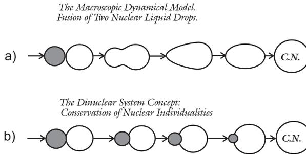
Fig. 6. The schematic illustration of the process of the compound nucleus formation in the complete fusion of two massive nuclei according to: (a) the macroscopic dynamical model [8], (b) the dinuclear system concept [11] (the figure from [11b]).
