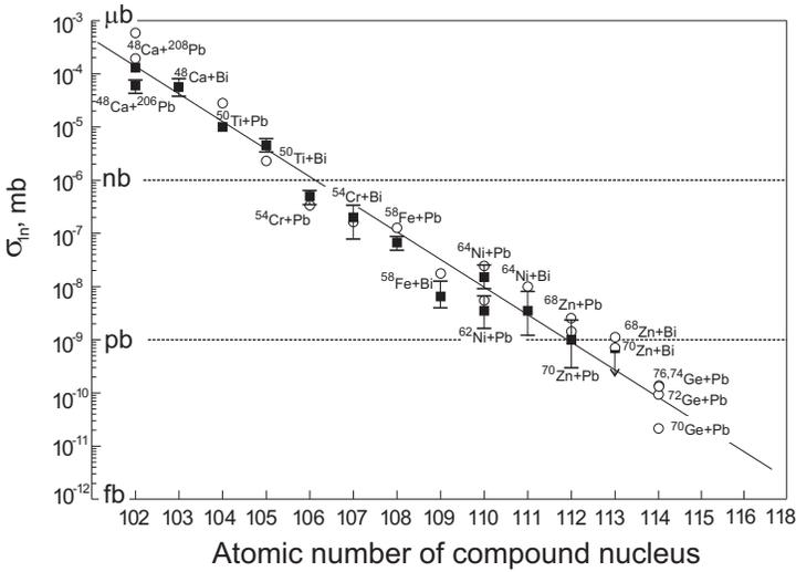
Fig. 12. Experimental data (black squares) and theoretical calculations (open circles) for the synthesis of elements from 102 to 114 in cold fusion reactions (HI,  $1n$ ) [27].
