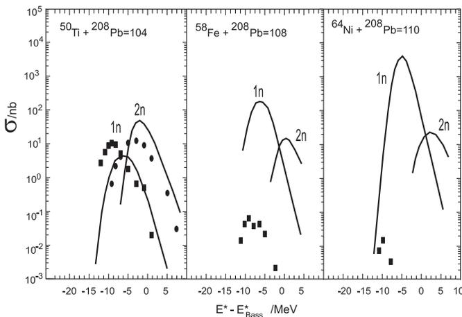
Fig. 1. The production cross sections of elements 104, 108 and 110 synthesized in cold fusion reactions (HI,1n,2n); points are experimental data [5], the curves — results of calculations [6].
