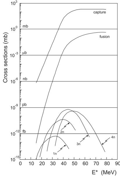
Fig. 15. The same calculations as in the Fig. 14 but for the synthesis of element 116 in the reaction  $^{248}\text{Cm} + ^{48}\text{Ca}$  [28].
