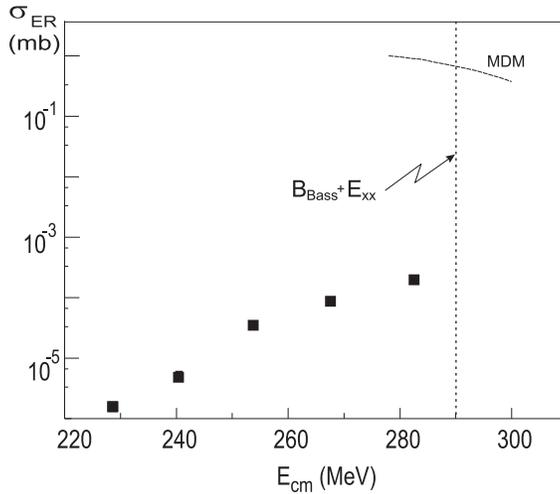
Fig. 5. The evaporation residue cross sections in the reactions  $^{110}\text{Pd} + ^{110}\text{Pd}$ ; squares are the experimental data, the curve is the result of calculation with using the MDM [11b].
