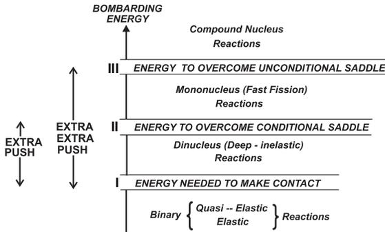
Fig. 3. The systematic of nuclear processes which are realized in the collision of two massive nuclei [8].
