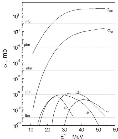
Fig. 14. The analysis of the reaction  $^{244}\text{Pu} + ^{48}\text{Ca}$  in the framework of the DNS-concept:  $\sigma_c$  — the capture cross section,  $\sigma_{\text{fus}}$  — the fusion cross section, curves with indices  $1n, 2n, 3n, 4n$  are the production cross section of different isotopes of element 114 [27].
