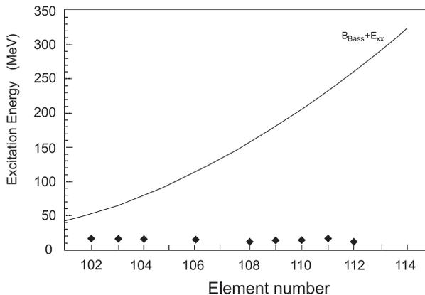
Fig. 4. The excitation energy of compound nuclei of 102 – 112 elements synthesized in cold fusion reactions (HI,1n); diamonds are experimental data [9], the line is the result of calculations with using the MDM [10].
