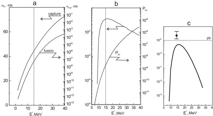
Fig. 13. The analysis of the reaction  $^{208}\text{Pb}+^{86}\text{Kr}$  in the framework of the DNS-concept [23]: a — the capture and fusion cross sections; b — the energy dependence of the factor  $P_{cn}$  and the ratio of  $\Gamma_n/\Gamma_f$ ; c — the energy dependence of the production cross section of element 118; the point is experimental data obtained in [24].
