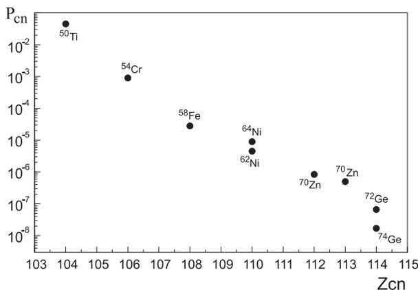
Fig. 11. The probability of complete fusion  $P_{cn}$  in cold fusion reactions calculated in the framework of the model using the Kramers type stationary solution to the Fokker-Planck equation [18].
