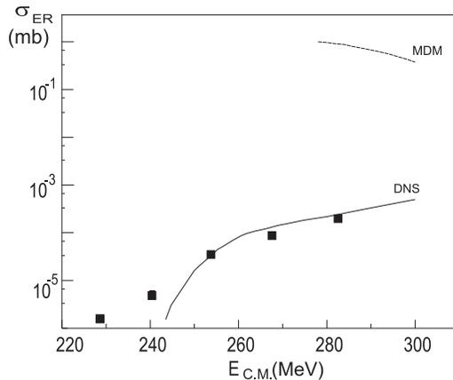
Fig. 9. The evaporation residue cross section in the reaction  $^{110}\text{Pd} + ^{110}\text{Pd}$  calculated by using the DNS-concept (solid line) and the MDM (dashed line) [11b].
