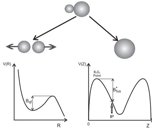
Fig. 8. Two ways of evolution of a massive DNS. The nucleus–nucleus potential (left) and potential energy of DNS (right) are indicated [11b].
