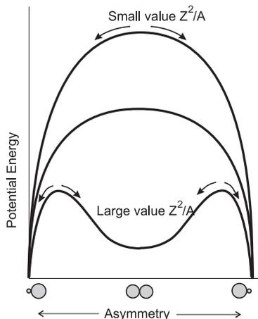
Fig. 2. The potential energy of two touching nuclear liquid drops in dependence of the parameter  $Z^2/A$  and mass asymmetry [7].
