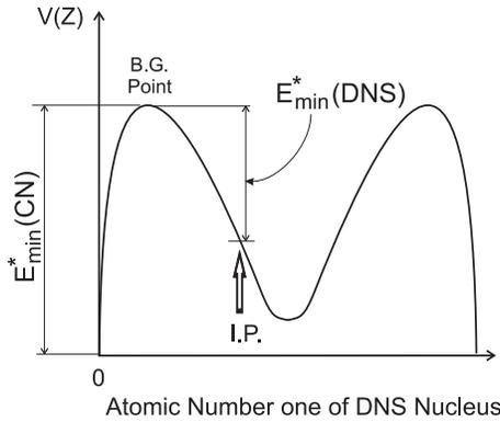
Fig. 16. The minimum of the excitation energy of the DNS necessary for complete fusion of two massive nuclei and the minimum value of the compound nucleus excitation energy according to the DNS-concept [11c].
