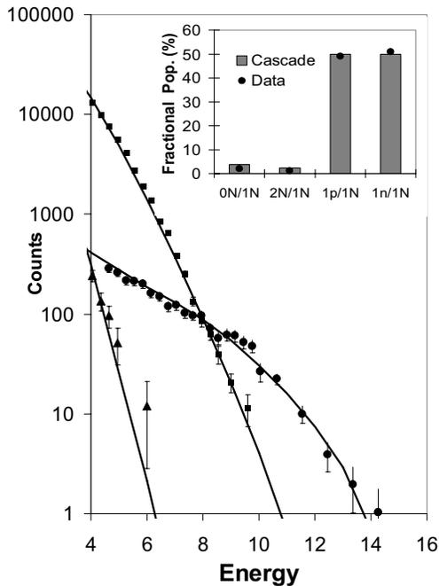
Fig. 2. The high-energy  $\gamma$ -ray spectra associated with the 0-, 1- and 2-nucleon emission channels (filled points, squares and triangles, respectively) are shown in comparison with statistical model calculations as described in the text. In the inset the measured fractional populations of the different residual nuclei are shown in comparison with the best fitting statistical model predictions.
