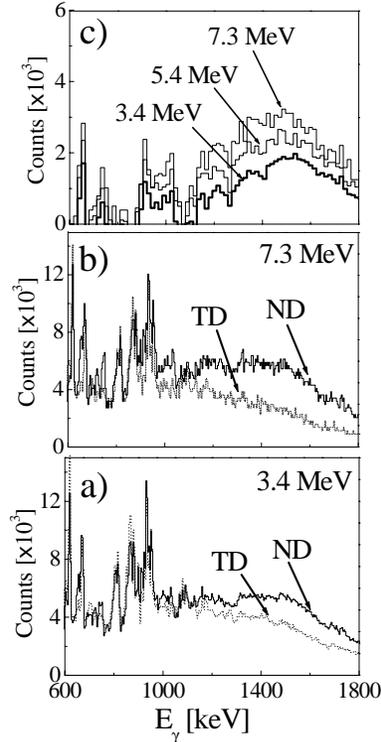
Fig. 4. Spectra of  $^{143}\text{Eu}$  collecting the entire decay flow (ND) and the triaxial contribution only (TD), gated by high-energy transition with  $\langle E_\gamma \rangle = 3.4$  (panel (a)) and 7.3 MeV (panel (b)). The intensity of the E2 bump observed in the ND spectra, obtained as a difference between the ND and TD spectra and normalized to the intensity of the 553 keV low spin spherical transition, is shown in the top part of the figure.
