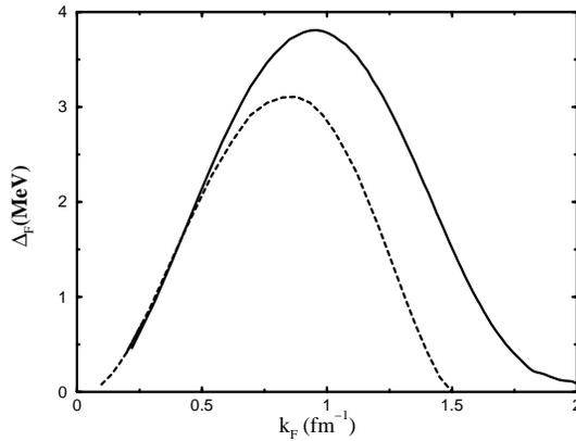
Fig. 1. Pairing gap at the Fermi energy,  $\Delta_F$ , calculated in neutron matter as a function of Fermi momentum, for the Gogny potential (solid line) and the Argonne potential (dashed line).
