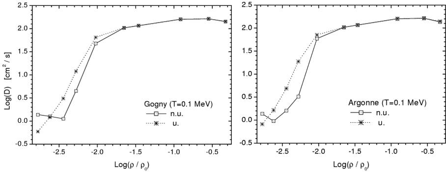
Fig. 4. Thermal diffusivity for inner crust matter calculated at  $T = 0.1$  MeV. The solid line represents the case of non-uniform neutron matter with nuclear impurities, while the dashed line is the standard uniform neutron matter. The symbols represent the zones where the calculation has actually been performed.
