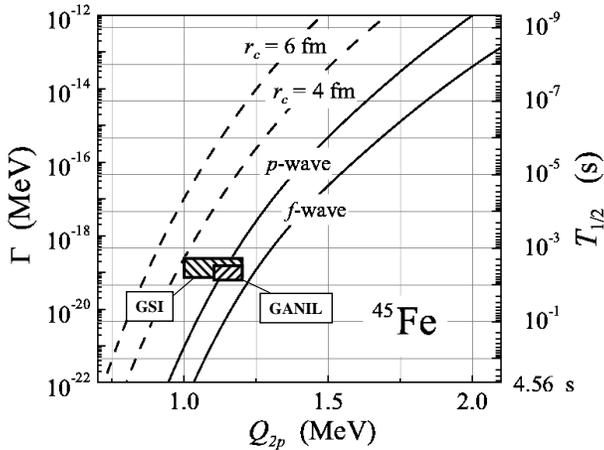
Fig. 4. Theoretical estimates of the partial half-life for the ground-state  $2p$  decay of  $^{45}\text{Fe}$ . The experimental values are indicated by the hatched boxes.
