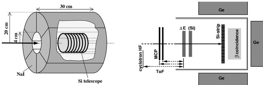
Fig. 1. Schematic drawings of the implantation setups used in the GSI experiment (left) and in the GANIL experiment (right).
