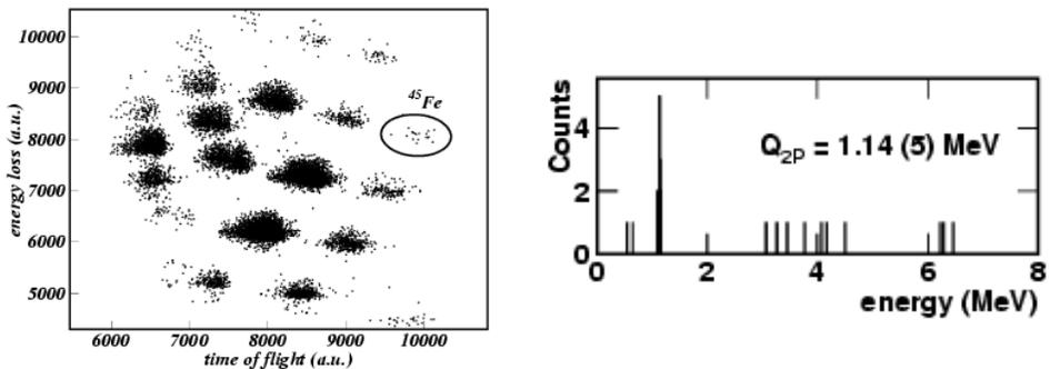
Fig. 3. Left: identification plot for ions stopped in the Si strip detector during the  $^{45}\text{Fe}$  measurement at GANIL. Right: decay energy spectrum correlated with the  $^{45}\text{Fe}$  implantation. Only events occurring up to 100 ms after implantation were considered.
