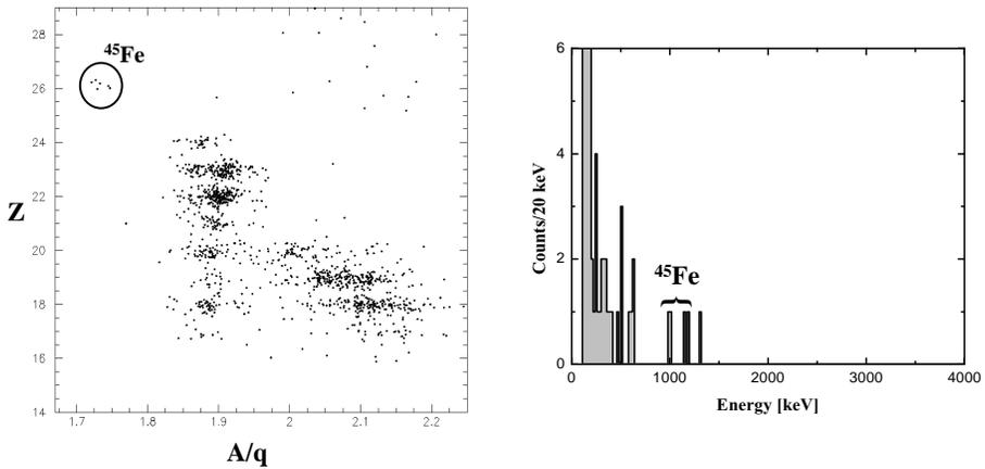
Fig. 2. Left: identification plot of ions which entered the Si telescope and triggered the DGF acquisition during the  $^{45}\text{Fe}$  measurement at GSI. Right: singles spectrum of all decay-like events anticoincident with the NaI detectors recorded during the whole run.
