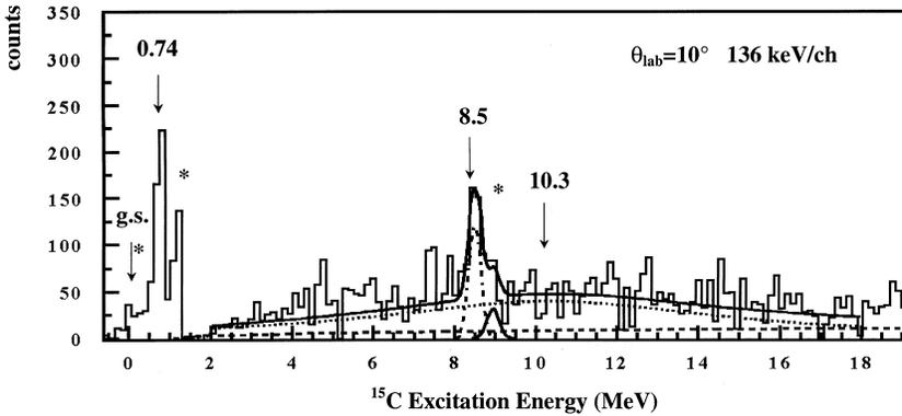
Fig. 1. Excitation energy spectrum of  $^{15}\text{C}$  at 57 MeV and  $10^\circ$ . Curves regarding fit in the continuum are visualized; dashed line is 3-body phase space contribution as given in Ref. [8]; the dotted line is the fit of the resonance at 10.3 MeV; the structure at 8.5 MeV has been modelled with two Gaussians (see text); the full thick line is the convolution of all the previous curves.
