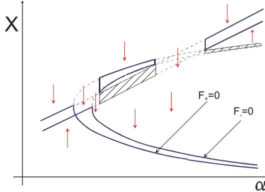
Fig. 4. Stochastic bifurcation diagram, corresponding to Eq. (3) with bounded noise. The arrows indicate the direction of the flow (see the text for an explanation of the meaning of the different regions).
