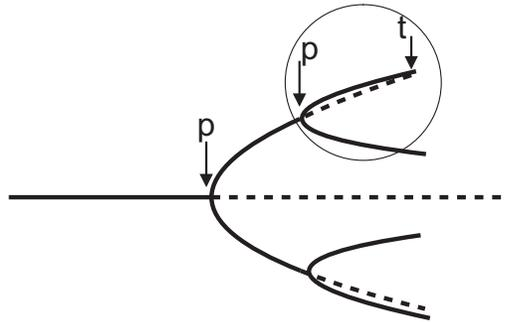
Fig. 3. Schematic view of a deterministic bifurcation diagram, showing one primary and two secondary bifurcations (within the circle). The symbols  $p$  and  $t$  indicate pitchfork and transcritical, respectively.
