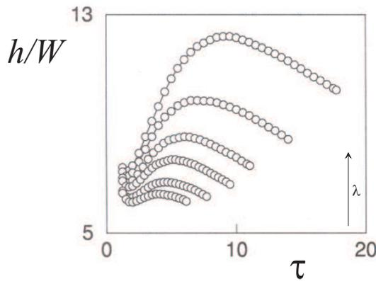
Fig. 2.  $h/W$  (the quality factor of the RTDF) *versus*  $\tau$ . The different curves are (from bottom to top) for increasing values of  $\lambda$ , as indicated by the vertical arrow. The resonance-like behavior increases when moving into the oscillatory region.
