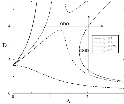
Fig. 7. Phase diagram for  $\alpha = -0.75$  and different values of  $p_+$ . Two distinct reentrant phase transitions, DOD and ODO, are indicated by the arrows.
