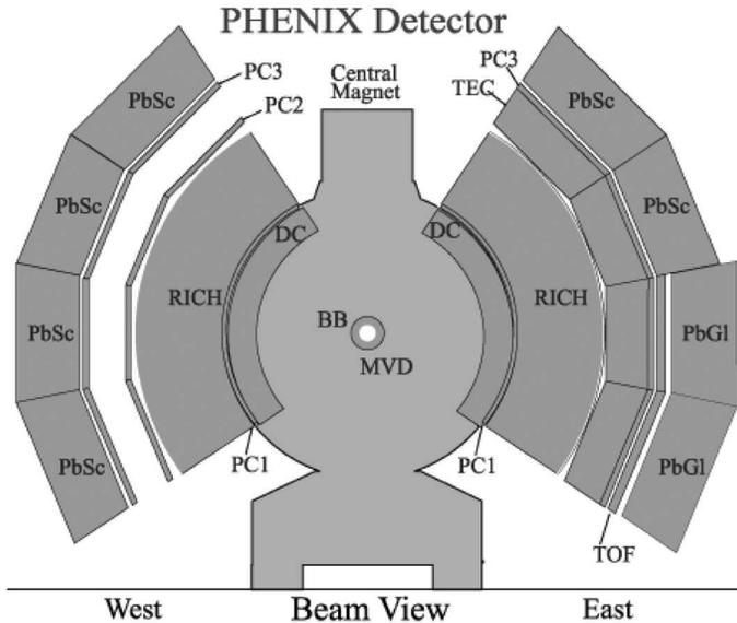
Fig. 2. The PHENIX experiment at RHIC (beam view).
