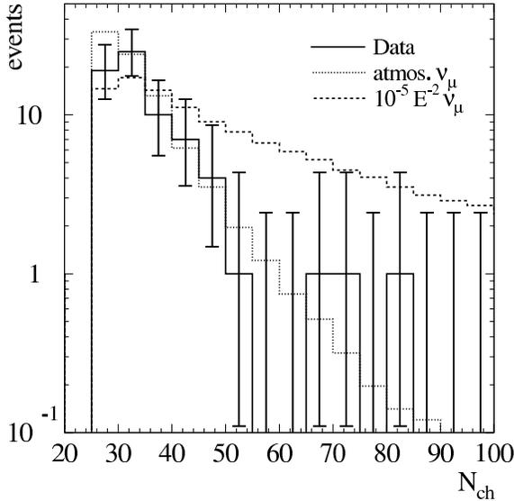
Fig. 3. Distribution of the number of hit PMTs ( $N_{\text{ch}}$ ) for the selected up-going muon events. In addition simulations for atmospheric neutrinos and AGN neutrinos, assuming a spectrum of  $d\phi/dE = 10^{-5}E^{-2} \text{ cm}^{-2}\text{s}^{-1}\text{sr}^{-1}\text{GeV}$ , are illustrated.
