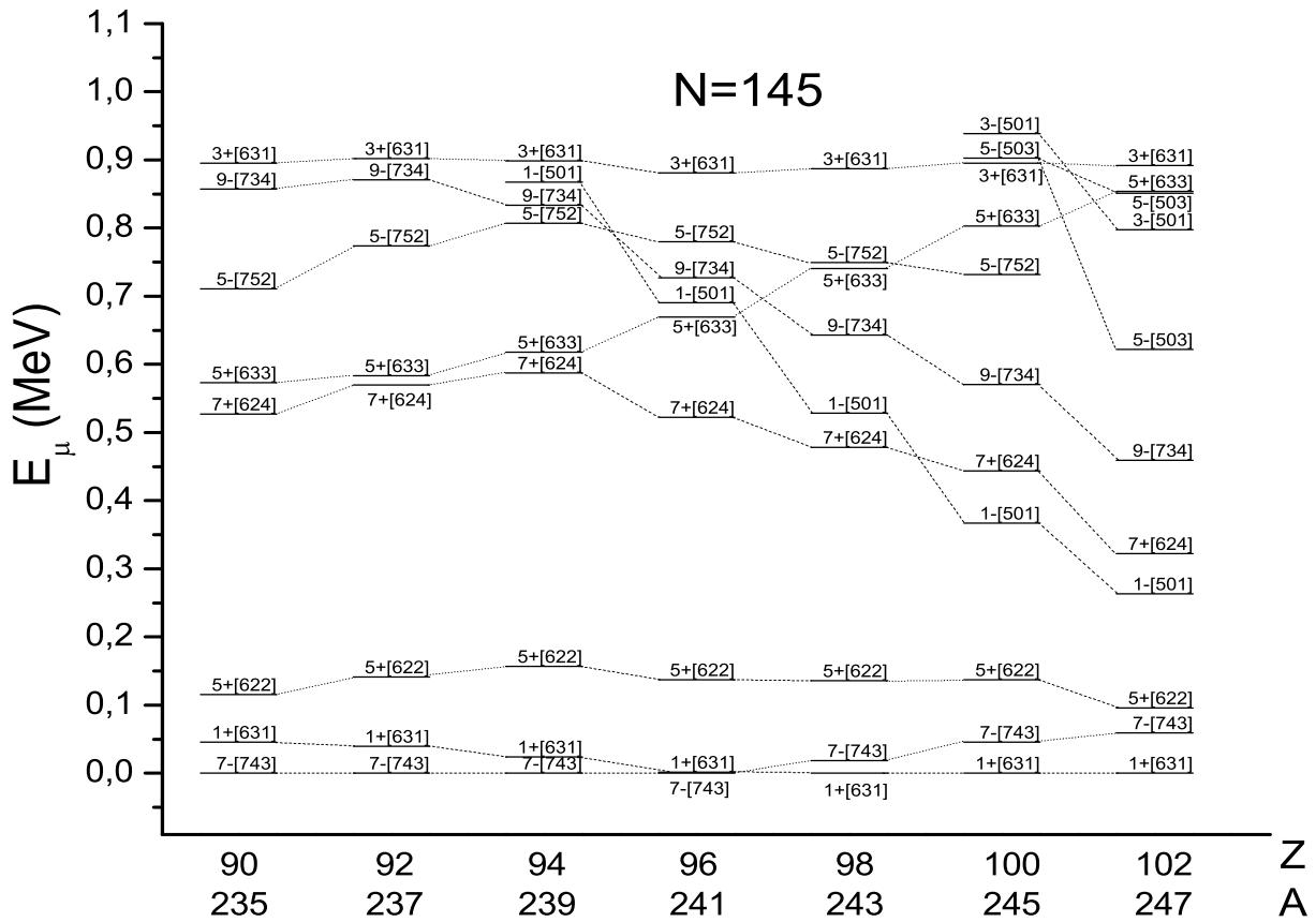
Fig. 3. Systematics of one-quasiparticle neutron states calculated for odd- $A$  isotones with neutron number  $N = 145$ .
