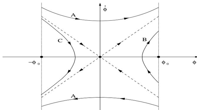
Fig. 4. Phase space trajectories of the uniformly impacting pendulums.
