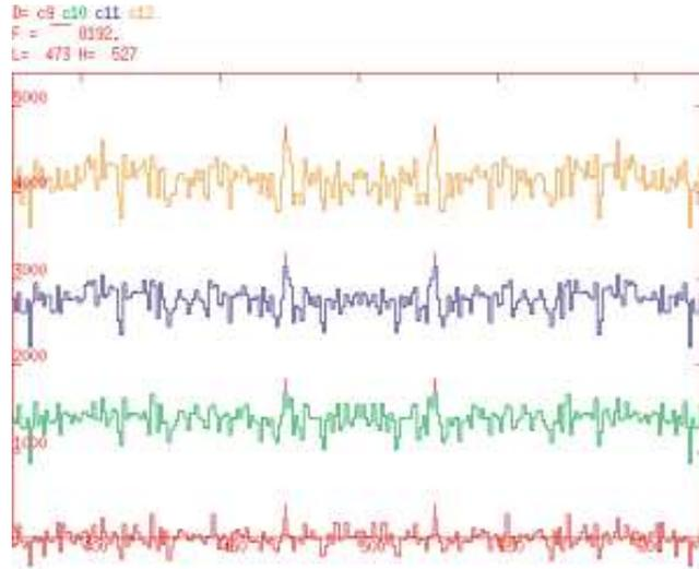
Fig. 7. Differences of perpendicular cuts, 204 keV wide, at 1440 keV across rotational planes with  $\delta = 12$  keV from data measured at 261 and 255 MeV beam energy for  $^{126}\text{Ba}$ . The four spectra, from bottom to top, are for thresholds of 22, 24, 26 and 28 on the coincidence fold [21].
