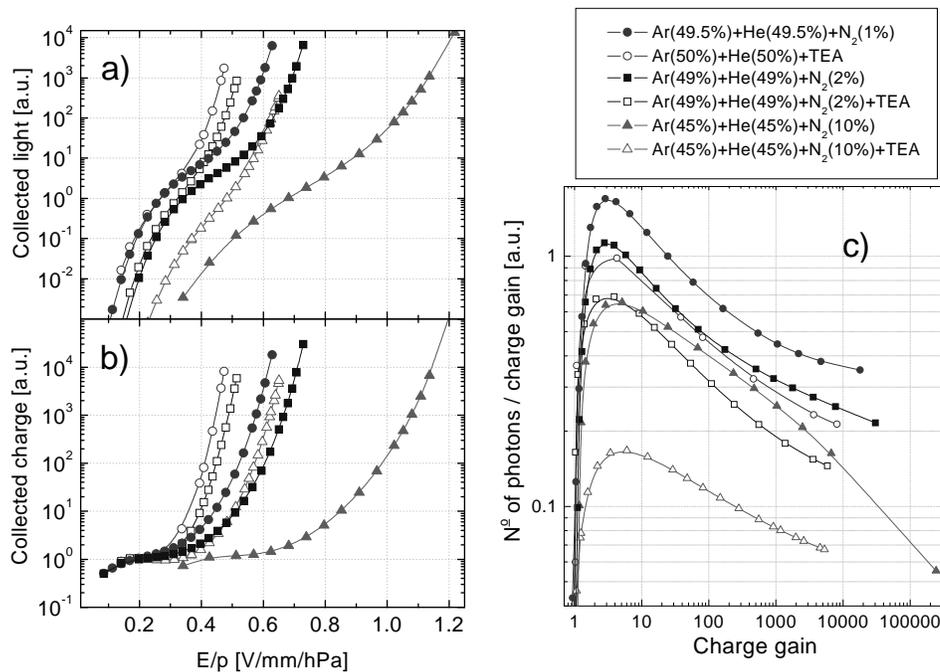
Fig. 2. Properties of selected gas mixtures measured in a test chamber with a 3.5 cm thick amplification gap: (a) the light yield from electron avalanches as a function of the reduced electric field in the gap, (b) the electron charge gain as a function of the reduced electric field, (c) the number of photons per single electron as a function of the charge gain.
