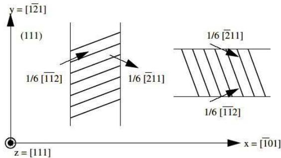
Fig. 1. Projections on the (111) plane of a generic fcc crystal of the system geometry for an edge (left) and screw (right) dislocation. Arrows denote Burgers vectors of partials. The area enclosed by the dislocation lines of the partials represents the stacking-fault ribbon.
