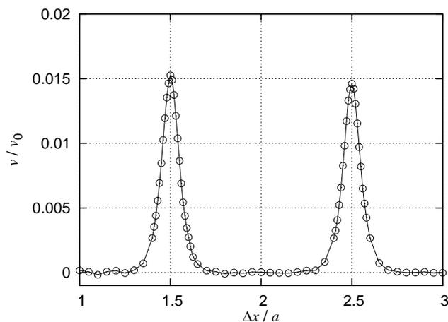
Fig. 3. Asymptotic rescaled average velocity  $v/v_0$ , with  $v_0 = f/\eta$ , obtained from 2000 trajectories, for an external tilt  $f = 1.9$  and a coupling constant  $K = 10$ , for different values of the rescaled equilibrium distance  $\Delta x/a$  between the particles. Peaks are located at distances equal to half-integer multiples of the period  $a$ .
