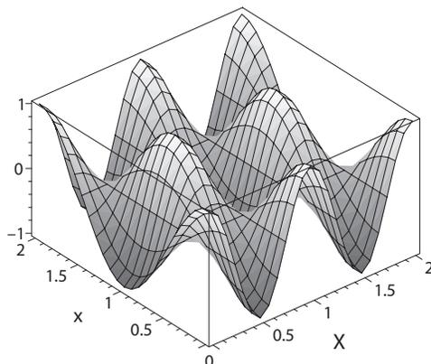
Fig. 2. Peierls potential  $V(X, x) = A_0 \cos(kx/2) \cos(kX)$  in the  $X$ - $x$  plane. The total potential (for zero tilt) is obtained by adding the  $x$ -dependent interaction potential, which is of the form  $K(x - \Delta x)^2/2$  in the harmonic approximation, see text for details. Notice that the system can move along the  $X$  direction going round the potential barriers, rather than overcoming them across the steepest paths as in the one-dimensional case.
