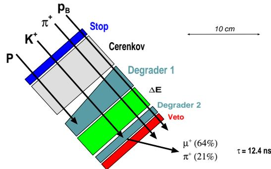
Fig. 3. A schematic top view of one telescope. It is composed of a stop, Cerenkov,  $\Delta E$  and veto scintillator and two degraders. The degraders are designed to stop protons in the first and kaons in the second one. Kaon decay products are registered in the veto counters with characteristic delay time. The ranges of pions, kaons and protons originating from the target and scattered protons ( $p_B$ ) with the same time-of-flight as kaons are indicated.
