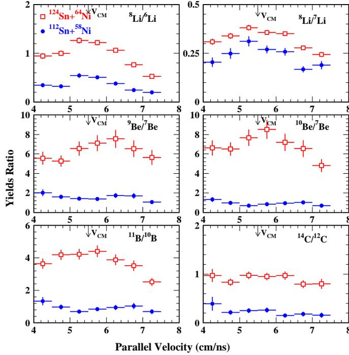
Fig. 1. The heavy-to-light isotope ratio for IMFs of  $3 \leq Z \leq 6$  as a function of their parallel velocity for the neutron rich (open squares) and neutron poor (solid circles) systems. The velocity integration bins are indicated by the horizontal error bars.
