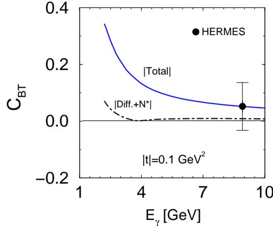
Fig. 1. The absolute values of beam-target asymmetry calculated without the  $s\bar{s}$ -knockout (dot-dashed curve) and with the  $s\bar{s}$ -knockout process (solid line) as a function of  $E_\gamma$  at  $|t| = 0.1$  GeV<sup>2</sup>. The data point is taken from Ref. [12]. The formulation for the calculations are given in Refs. [11, 13, 14]. Note that the nearly pure  $s\bar{s}$  wave function for the  $\phi$  meson and the  $s\bar{s}$  content of 1% in the proton are assumed.
