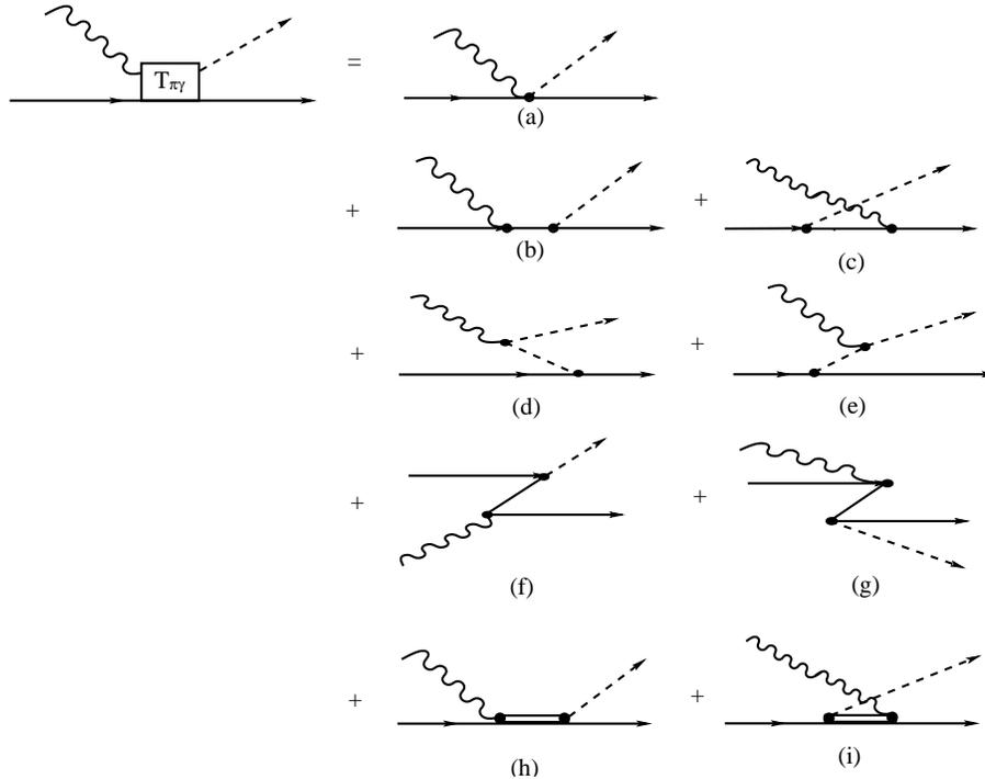
Fig. 1. The tree-level Feynman diagrams for  $\gamma N \rightarrow \pi N$ : (a) the Kroll–Rudermann graph, (b) and (c) the two time-ordered contributions to the direct and crossed nucleon pole graph, (d) and (e) the two time-ordered contributions to the pion pole graph, (f) and (g) the Z-graphs and (h) and (i) the  $\Delta(1232)$  resonance graphs. A solid, dashed and wavy line represents a nucleon, pion and photon, respectively.
