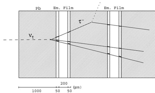
Fig. 1. The schematic structure of an ECC cell with the  $\nu_\tau$ CC interaction.
