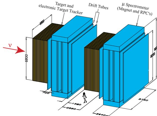
Fig. 2. The schematic view of the OPERA detector.
