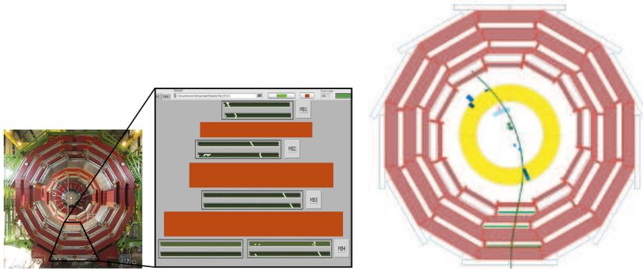
Fig. 8. Muon data recorded in CMS DT chambers without magnetic field (left). On the right, an event display taken end of August with a field of 3.80 Tesla during the Cosmic Challenge and showing active muon, HCAL, ECAL and Tracker detectors.
