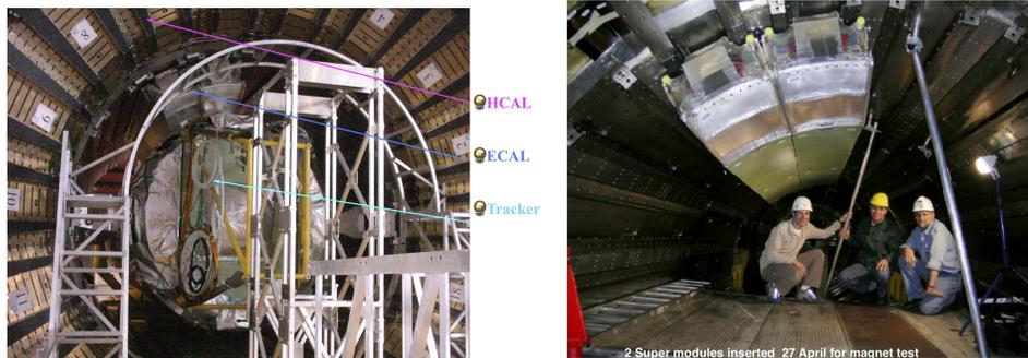
Fig. 6. HCAL, ECAL and Tracker elements installed inside the magnet for the Cosmic Challenge (left). Two ECAL SM inserted into the HCAL (right).
