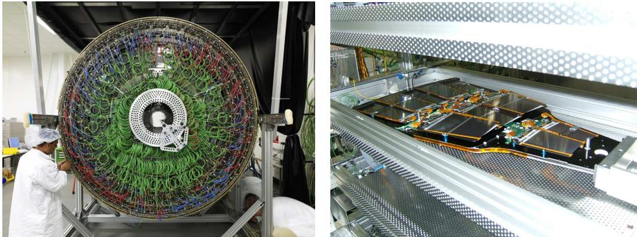
Fig. 13. The completed Tracker Inner Barrel (left), a TEC petal (right).
