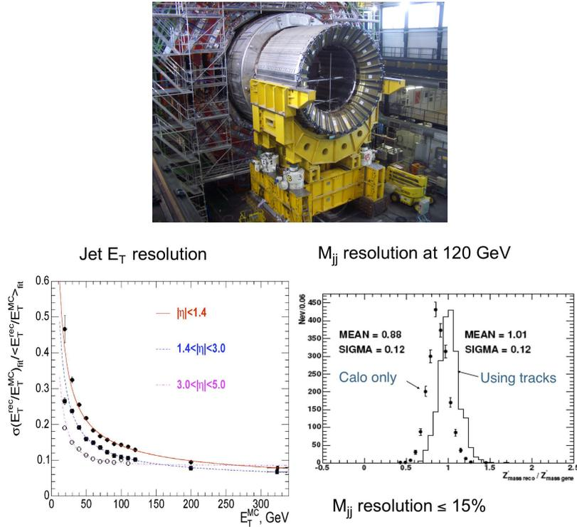
Fig. 10. Half barrel HCAL insertion into the magnet coil (top). Jet  $E_T$  and mass jet-jet resolutions (bottom).
