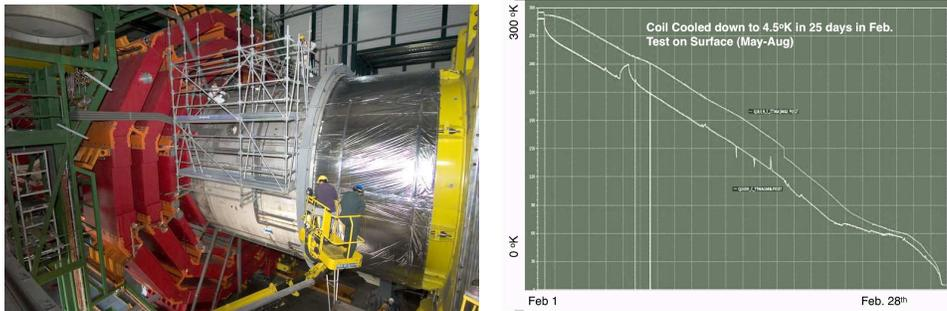
Fig. 5. The coil insert (left) in the vacuum tank supported by YB0 and the coil cool-down curve (right).
