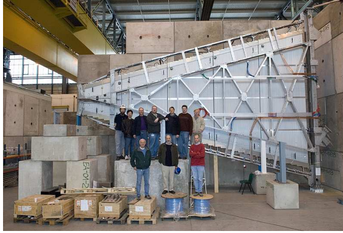
Fig. 8. Pre-assembled “Big Wheel” MDT sector for the end-caps.
