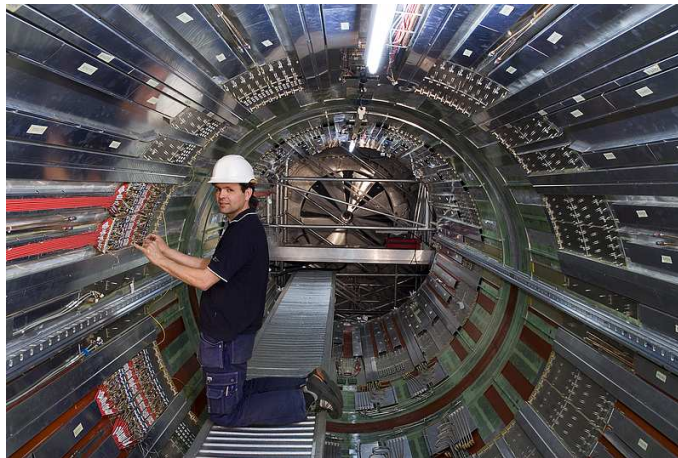
Fig. 10. Services (cables and pipes) for the ID installed along the inner wall of the barrel LAr cryostat.
