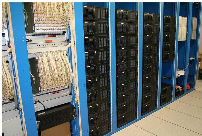
Fig. 9. Barrel LAr readout electronics and DAQ system in the underground counting room.
