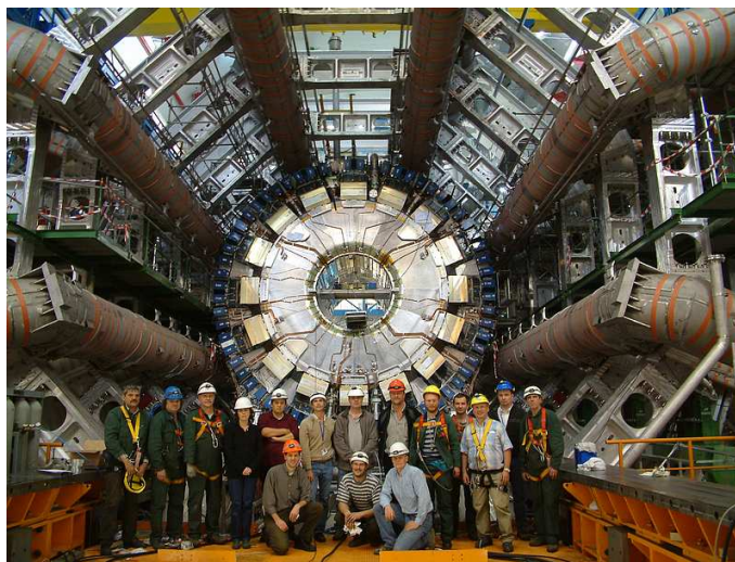
Fig. 5. Placement of the integrated barrel LAr and Tile Calorimeter into the detector centre, inside the coils of the Barrel Toroid (4th November 2005).
