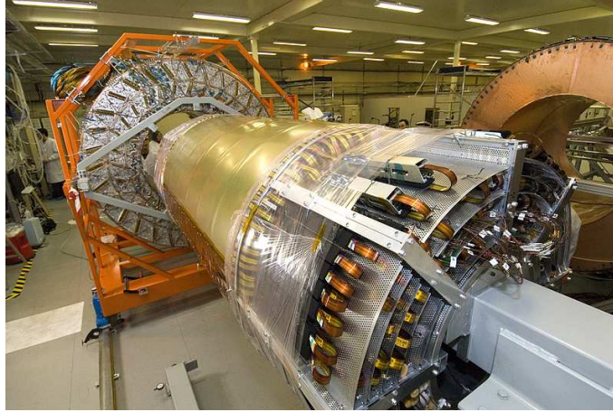
Fig. 3. Integration of the barrel ID: insertion of the SCT into the TRT (Feb. 2006).
