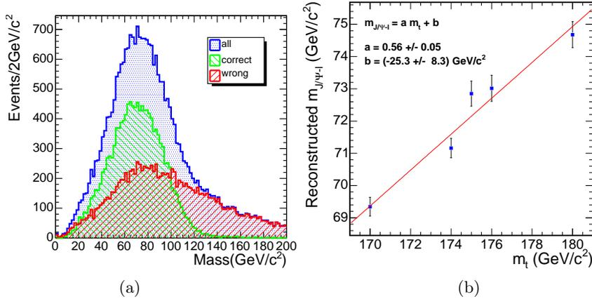
Fig. 4. (a) Three-lepton invariant mass distribution for  $m_t = 175 \text{ GeV}/c^2$  for selected events. (b) Correlation between the reconstructed three-lepton invariant mass and the input top mass.
