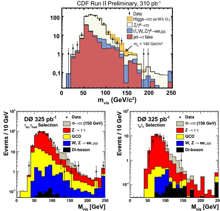
Fig. 5. Distribution of the visible mass  $M_{\text{vis}}$  for the analysis by CDF (top), and the two options considered by DØ : the one involving hadronic tau decays (bottom left) and one with the  $e\mu$  final state (bottom right). Data are compared to the predicted background from the SM and a possible signal.
