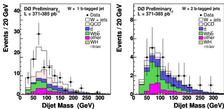
Fig. 1. Dijet invariant mass in the  $W+2$  jet events having one tagged  $b$ -jet (left) or both of them  $b$ -tagged (right) in the Higgs search by the  $D\bar{O}$  Collaboration. Data (crosses) are compared to the background predictions (stacked histograms).
