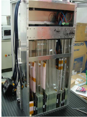
Fig. 5. Picture of the ARM2 LHCf calorimeter. The outside dimensions are 90 mm width, 300 mm length and 600 mm height. The light from the scintillator plates is guided by light fibres to the Hamamatsu photomultipliers. The black rectangular boxes house the silicon detector modules.
