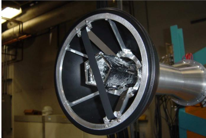
Fig. 6. A view of the 1/2 inch tape traversing the delrin hemisphere. The 10 element half of the SCEPTAR beta detector lies directly behind the tape. The tape system (MTC), not shown, was constructed at LSU.
