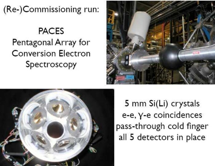
Fig. 10. The conversion electron spectrometer PACES, constructed at LSU, is shown mounted at the center point of the  $8\pi$  spectrometer (upper photo — see also Fig. 5). The 5 Si(Li) detectors are shown mounted (lower photo) in the LN<sub>2</sub> cryostat inside the delrin hemisphere. The beam travels through the hollow *cold-finger* to be deposited on the tape (not shown) at the focal point of the Si(Li) array.
