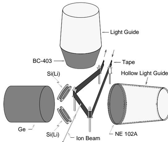
Fig. 1. Sketch of the spectrometer system constructed at LSU that was used in the  $^{74}\text{Rb}$  branching ratio experiment.
