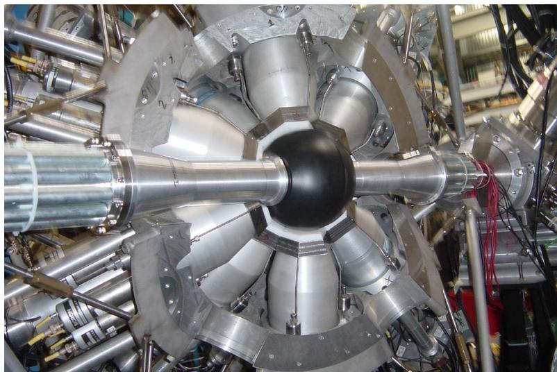
Fig. 5. A view of the  $8\pi$  opened showing half of the array and the beamline with the black delrin sphere at the center. The sphere separates at the *O-ringed* equator (which lies in a vertical plane) so that the left half can be moved out of the  $8\pi$  array.
