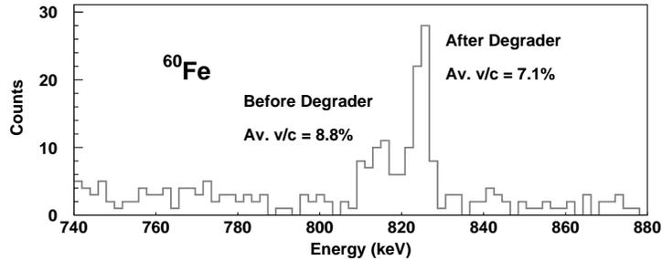
Fig. 4. Excerpt of spectrum corresponding to the 824 keV ( $2^+ \rightarrow 0^+$ ) transition in  $^{60}\text{Fe}$ , measured at the CLARA-PRISMA RDDS setup with the  $^{64}\text{Ni}$  (400 MeV) +  $^{208}\text{Pb}$  reaction. The two components with different average velocities are indicated.
