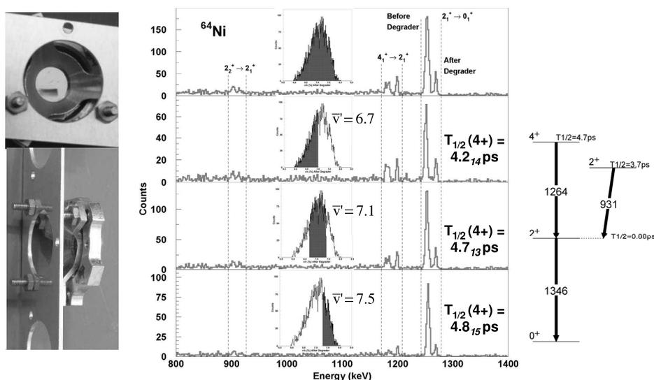
Fig. 3. The left panel shows a picture of the target-plunger device developed at IKP-Universität zu Köln. The right panel shows the RDDS spectra for 150  $\mu\text{m}$  for the inelastic channel of  $^{64}\text{Ni}$  with different  $\bar{v}$  conditions on the velocity (and therefore energy) of the recoil.
