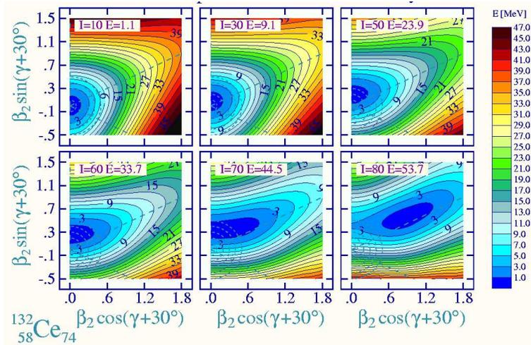
Fig. 1. Total macroscopic energies according to LSD method in the  $\{\beta, \gamma\}$  plane. The energies are normalised to  $E_{\text{lsd}}(0)$ . At each point and for each spin the energy has been minimized over  $\alpha_{4,0}$ ,  $\alpha_{6,0}$ ,  $\alpha_{8,0}$ .
