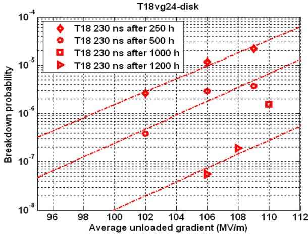
Fig. 6. Accelerating gradients in unloaded 12 GHz CLIC structure [9]. Goal is the nominal breakdown rate below  $3 \times 10^{-7}$ .
