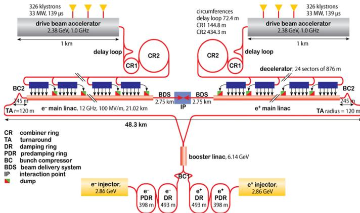
Fig. 3. Schematic layout of CLIC 3 TeV (not to scale).
