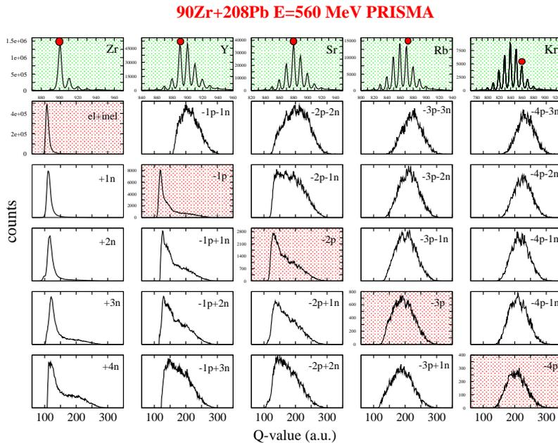
Fig. 3. TKEL spectra obtained in the reaction  $^{90}\text{Zr}+^{208}\text{Pb}$  for the indicated transfer channels. In the top row are shown the mass distribution associated to the different nuclear charges, while the circles indicate the specific masses corresponding to the spectra displayed along the upper-left/lower-right diagonal. The centroid of the elastic+inelastic channel corresponds to  $Q = 0$ . The scale of the  $Q$ -value axis is 1 MeV/channel.
