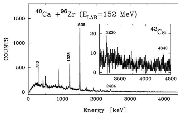
Fig. 2.  $\gamma$ -ray spectrum with expanded region in inlet for  $^{42}\text{Ca}$  obtained in the  $^{40}\text{Ca}+^{96}\text{Zr}$  reaction.
