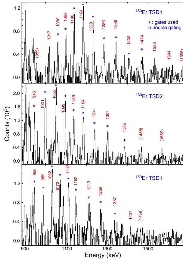
Fig. 6. Background-subtracted coincident  $\gamma^3$  spectra illustrating the new high moment of inertia sequences observed in  $^{160}\text{Er}$  and  $^{159}\text{Er}$ .
