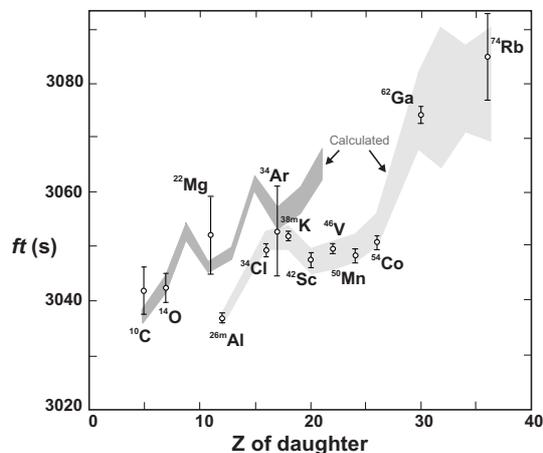
Fig. 3. Experimental  $ft$  values plotted as a function of the charge on the daughter nucleus,  $Z$ . Both bands represent the quantity  $\overline{F}t/((1 + \delta'_R)(1 - \delta_C + \delta_{NS}))$ . The two separate bands distinguish those beta emitters whose parent nuclei have isospin  $T_z = -1$  (darker shading) from those with  $T_z = 0$  (lighter shading).
