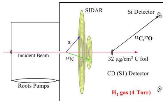
Fig. 2. Schematic of the experimental setup for the  $^{18}\text{F}(p, \alpha)^{15}\text{O}$  and  $^{17}\text{O}(p, \alpha)^{14}\text{N}$  studies.
