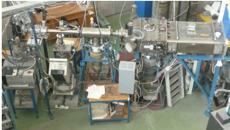
Fig. 3. The IGISOL device, based on a Scandinavian type isotope separator with an additional gas catcher ion guide.
