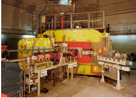
Fig. 2. The K_{\text{max}} = 160 heavy-ion cyclotron and the layout of the beam lines with the experimental stations. The upper part of the layout shows schematically the PET Radiopharmaceuticals Production Centre (see Sec. 4).
