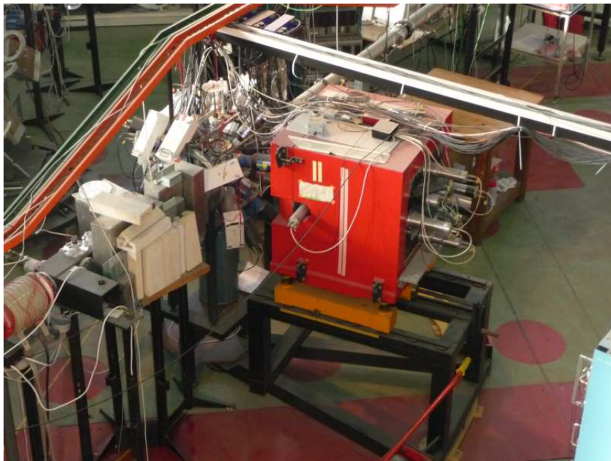
Fig. 5. JANOSIK, large NaI(Tl) crystal and its ancillary detectors for high-energy gamma ray studies.
