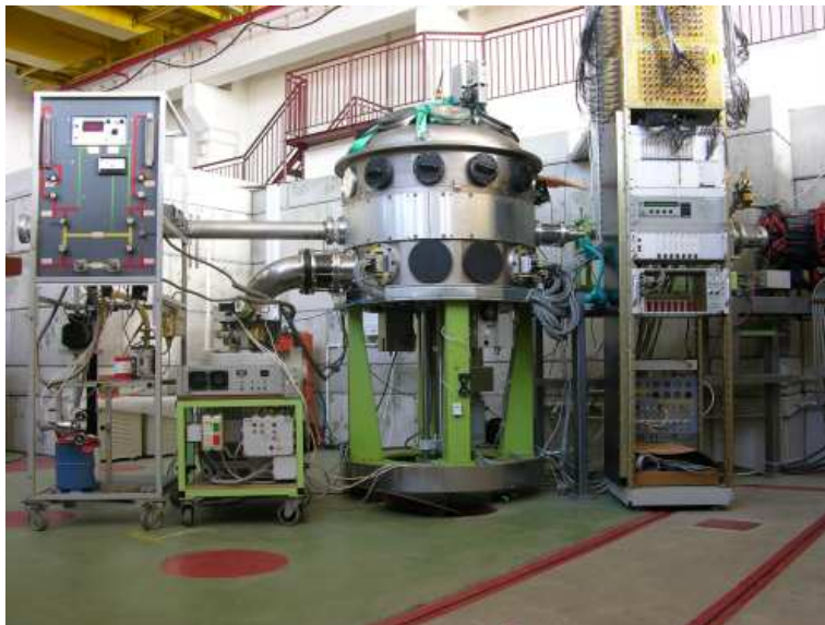
Fig. 6. The ICARE reaction chamber with vacuum and gas system.
