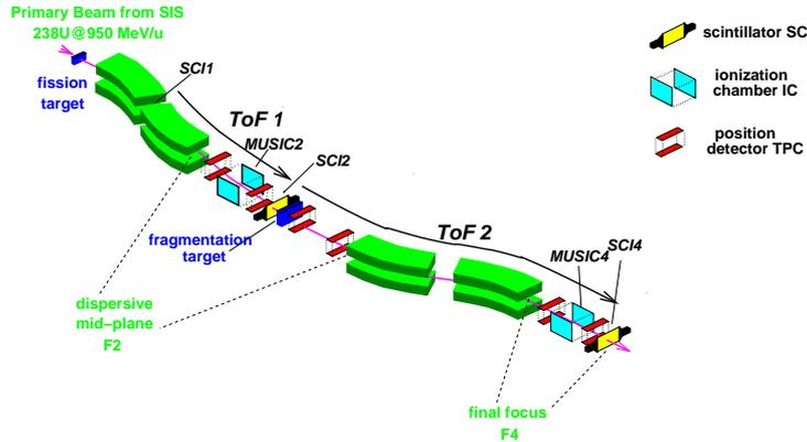
Fig. 1. Schematic layout of the FRS showing the dipole magnetic elements and the detection system used in the experiment.
