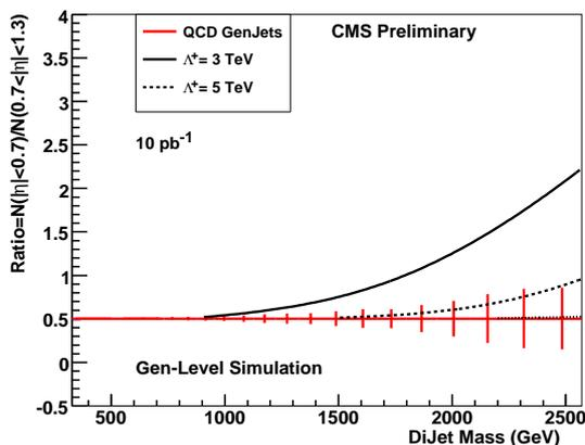
Fig. 2. Ratio of central to forward di-jet events as function of the di-jet invariant mass. The curves show the QCD prediction as well as the prediction for contact interactions for two scales. The error bars show the sensitivity for  $10 \text{ pb}^{-1}$ .
