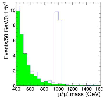
Fig. 1. Histograms of the  $\mu^+\mu^-$  invariant mass for  $1\text{ TeV}/c^2$   $Z'$  plus background (open histogram) and for background only (shaded histogram), at the event-generator level. The number of events per bin is normalised to an integrated luminosity of  $0.1\text{ fb}^{-1}$ .
