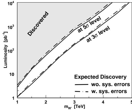
Fig. 8. Luminosity needed to make a  $5\sigma$  ( $3\sigma$ ) discovery of a  $W'$  in the decay channel  $e\nu$ .
