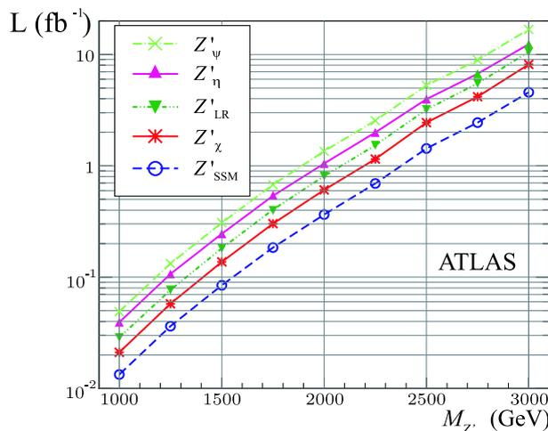
Fig. 7. Luminosity required for a  $5\sigma$  discovery of a  $Z'$  signal for various  $Z'$  models.
