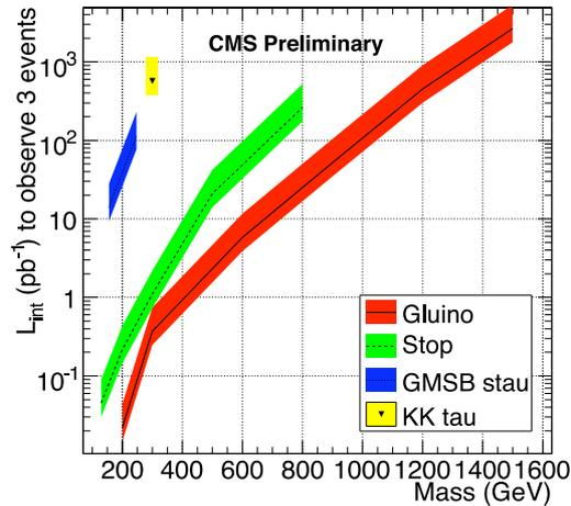
Fig. 14. Luminosity needed for a discovery requiring 3 events (for no background) for various heavy stable charged particles in CMS.
